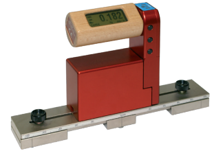
BlueLEVEL with a flexbase for steplength from 90 up to 240 mm
