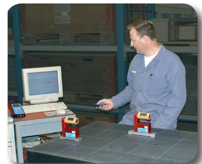
Flatness measurement with a measuring and reference instrument
