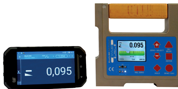
Outdoor smartphone with preinstalled BlueCLINO High Precision APP
